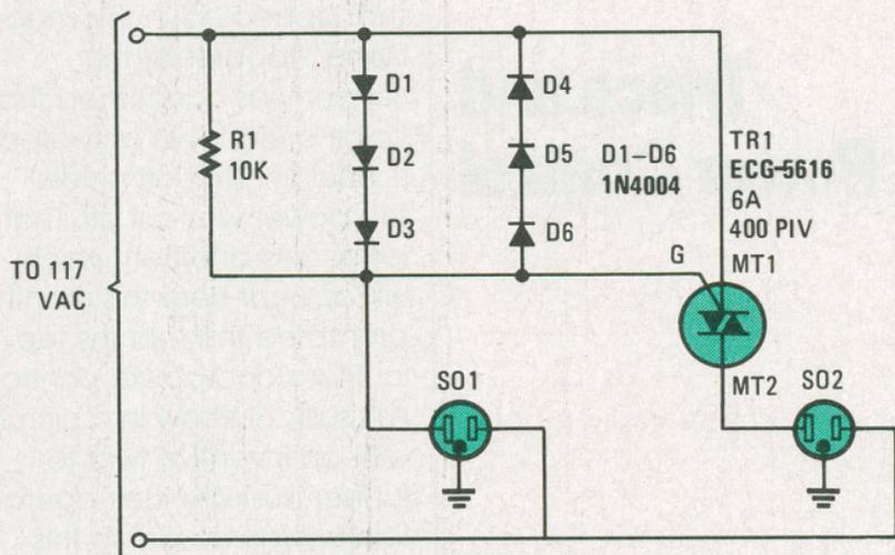
Fig. 4. This circuit to generate a trigger signal for a Triac looks odd, but it works very well. The diodes provide the Triac gate with a voltage-limited gate signal.
