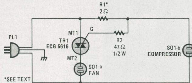
Fig. 6. When this Triac circuit senses current flow through S01-a, it activates the device plugged into S01-b. The values of the resistors must be chosen for the specific devices to be plugged in.
